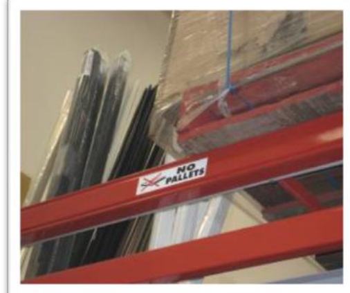
12. UNACCEPTABLE - Pallets cannot be placed on beams with 'No pallet' stickers.
