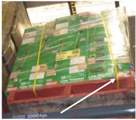
7. UNACCEPTABLE - Wrap not covering four corners of the pallet
