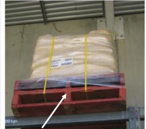
4. UNACCEPTABLE – a poor quality pallet strapped to a standard pallet
