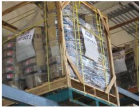
9. ACCEPTABLE – Non standard pallets (skids) are unable to be locked into racking but if they are stable with no risk of collapse can be strapped to another standard pallet.
