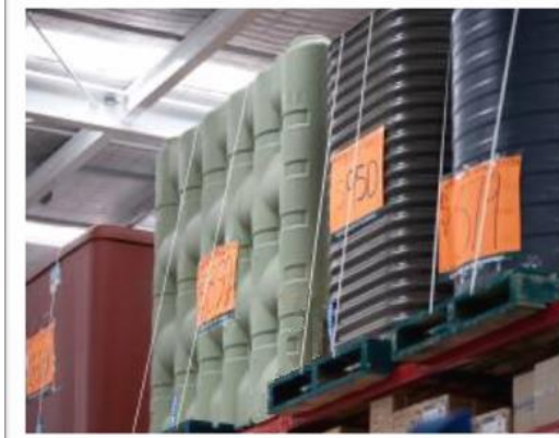
11. ACCEPTABLE - Single item products over 1.8 m can be placed in racking – they require strapping only
