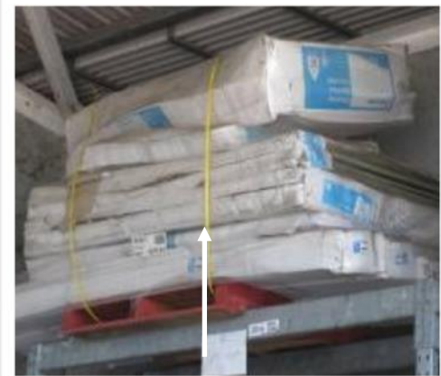
6. UNACCEPTABLE - Stock unbalanced, wrap not covering all stock or all corners of the pallet
