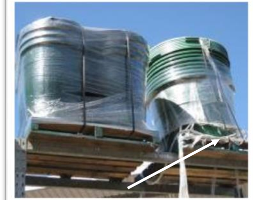
8. UNACCEPTABLE - Wrap deteriorated as a result of weather exposure
