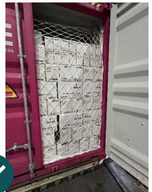
Figure 2 - Example of cargo nets in use
