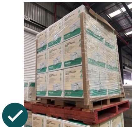
Figure 13 – Example of correct use of corner posts
