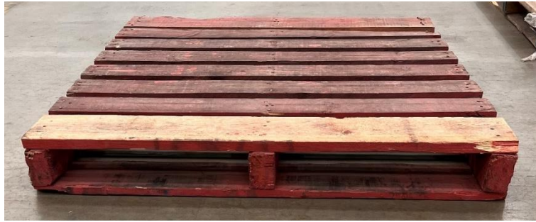
Figure 12 - Example of a wooden pallet made of solid timber
