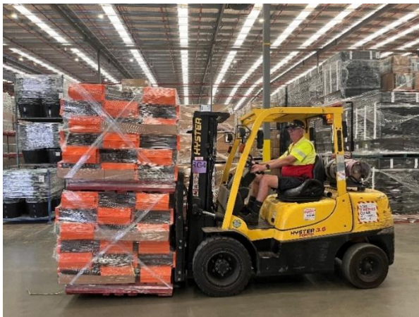
Figure 16. Height of the pallet should have clearances to allow for forklift and pallet jack tynes access.
