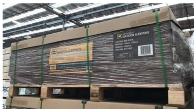
Figure 20. Example of a well labelled and packed timber pack
