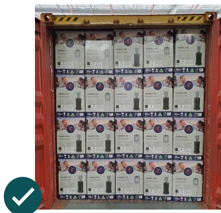
Figure 3 - Example of a well packed hand load container
