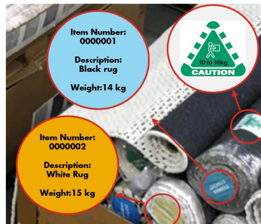
Figure 28. Each label is to include the item number, product description, weight and weight icons as clear identifiers.
