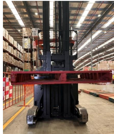
Figure 16. Height of the pallet should have clearances to allow for forklift and pallet jack tynes access.
