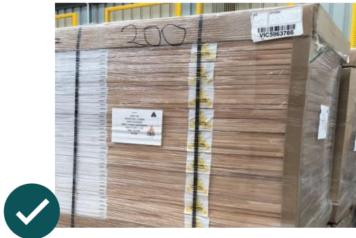
Figure 21. Proper cardboard top and corner pillar protection used
