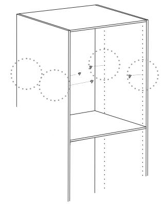
TIP! - You can use a spirit level to quickly find the corresponding holes at the same height.
