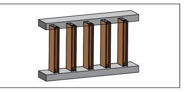
**STEP 4 - Install the Two-Piece Batten Bases**
