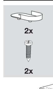
Align the hanger bracket lugs with the predrilled holes in the Left and Right Side Panels. Push the bracket and drive flush to the cabinet surface.
