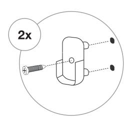
Note – If hanging heavy items, permanently fix the hanger brackets with the supplied screws.
