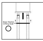
Place the base washer O-ring over the end of the hoses and insert into the base of the mixer.
