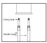
Firmly tighten the flexible hoses into the inlet tails at the base of the body, being careful to avoid damage to the O-ring seals. If the hoses have red and blue indicators make sure they are connected to the correct inlet port in the mixer.
