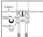
5. Position the fixing plate washer and fixing plate onto the bolt. The flexible hoses should be positioned towards the front of the sink/basin with the lever handle pointing towards the user. Fixing bolt positioned at the back.
