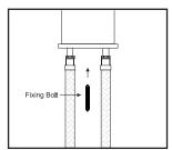
2. Screw the fixing bolt into the mixer base (remove fixing nut if installed).
