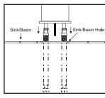
Feed the hoses through the sink/ basin hole, each end alternatively, and position the base washer between the sink/basin and the mixer base.
