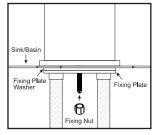
6. Lock the mixer onto the sink / basin by tightening the fixing nut onto the fixing plate.
