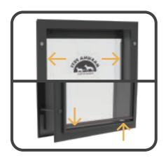
3. Insert/adjust flap position in frame
