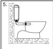
Securely connect the WC pan with the elbow pipe.
