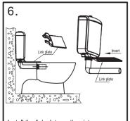
Install the link plate on the cistern.
