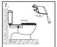
Measure and mark the area to be cut from the link plate by loosely installing the toilet seat into the pan. Remove both items and make the cut with a fine tooth hand saw/hacksaw. Note - Use the cut lines on the back of the link plate to ensure you achieve a straight cut. Reinstall the link plate.
