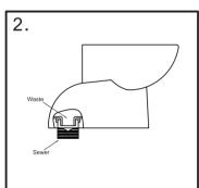
Connect the waste to the sewer, ensure that the sewer connection is connected correctly and that a good seal has been achieved.
