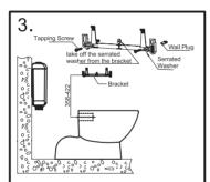
Hang the bracket on the wall. Note - Take caution when selecting the area to be drilled as water pipes or other hazardous objects may be present in wall. Install the cistern.
