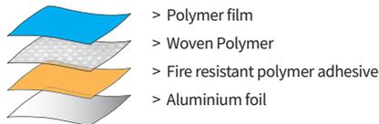
Ametalin utilises Advanced Laminating Technology; the polymer adhesive remains tacky indefinitely and provides superior resistance to heat, fire and delamination.
