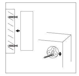
Place the cabinet brackets over the exposed screws, and slide downwards to lock into place.
