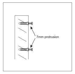
5. Install the screws into the wall plugs, leaving about 7mm protruding from the wall.
