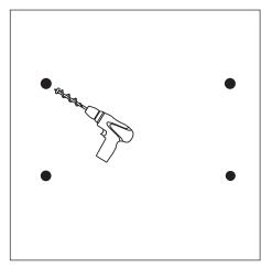
3. Drill into the marked out locations using an appropriate drill bit (i.e. masonry bit for tiles).
