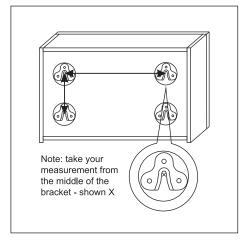
1. Take measurements from the back of the cabinet's fixing points.
