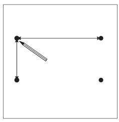
2. Mark out the fixing locations onto the wall.
