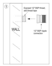
Apply thread tape before installing the 1/2" BSP nipple connection. NOTE- the spanner drive must be closest to the wall & finish flush.
