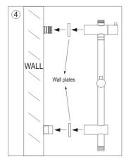
Install the exposed shower rail onto the 2 exposed wall fixing points. Lock into position using the grub screws & allen keys provided.
