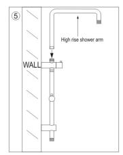
Insert the high rise shower arm onto the exposed rail. Ensure that the 2 rubber seals are engaged. Lock into position with the hand tighten locking nut. If a good seal is not achieved you can nip it up, but take care to protect the chrome from the tool being used.
