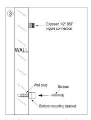
Install the bottom mounting bracket onto the wall using the wall plugs & screws provided ensure the appropriate drill bit is used for your wall.
