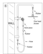
Connect the hose to the bottom of the exposed rail & to the hand piece using the rubber washers provided. Then connect the over head shower to the high rise shower arm using the rubber washers provided.
