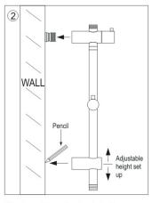
Mark out the desired bottom mounting brackets fixing location on the wall as shown in the diagram above.
