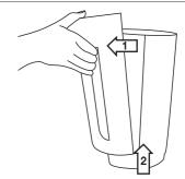
Remove the housing cover as shown (magnetic fastening). First detach the magnetic fastening at the top, and then at the bottom.
