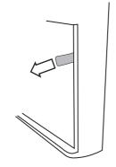
3. Pull out the pre-filter. Now, to pull out the combi filter, pull carefully on the side tabs.
