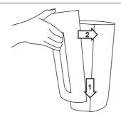
Re-insert the housing cover as shown until you see and hear it click into place (magnetic fastening). First attach the magnetic fastening at the bottom, and then at the top.
