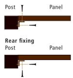
Fix to posts using suitable screws and easy screen brackets (available in the aisle with easy screen products) or direct to post just using screws.
