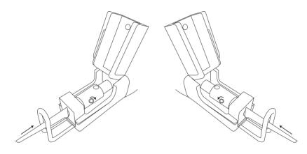
$4.\ Return$  blade cover to its original position, tighten the PH2 screw. The tool is now ready for operation.
