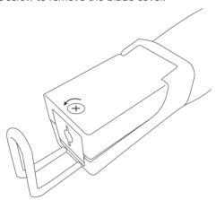
2. Lift the blade cover to expose the blade mounting system. Using a 4 mm Hex key loosen both grub screws.
