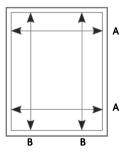
Measure inside the window frame at the top and the bottom of the frame to ensure the window frame is straight. In case you receive different readings, a smaller dimension should be considered.
