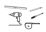
Spirit level, tape measure, pencil, drill, Phillips head screwdriver
