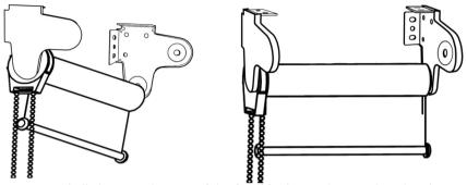
First insert ball chain mechanism of the first blind onto the matching bracket, then insert endplug with pin onto the opposite bracket.
