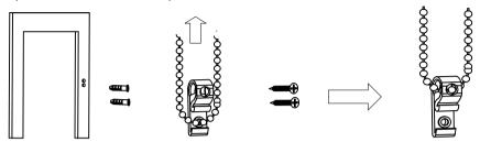
Install both tension devices using screws provided in the pack. Adjust position so that the chain can pass through device freely.
