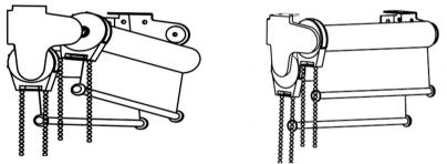
Insert ball chain mechanism of the second blind onto the matching bracket, then insert endplug with pin onto the opposite bracket.
