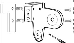
Fix the brackets using screws included and a drill or a Phillips head screwdriver.
