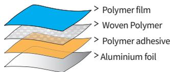
Ametalin utilises Advanced Laminating Technology; the polymer adhesive remains tacky indefinitely and provides superior resistance to heat, fire and delamination.
