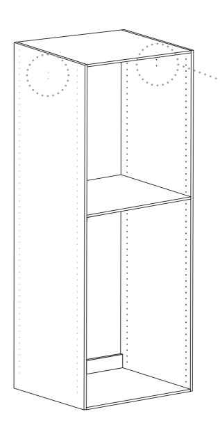
TOP 1536mm and 2048mm Cabinet Shells include additional holes for Hangrail installation.
