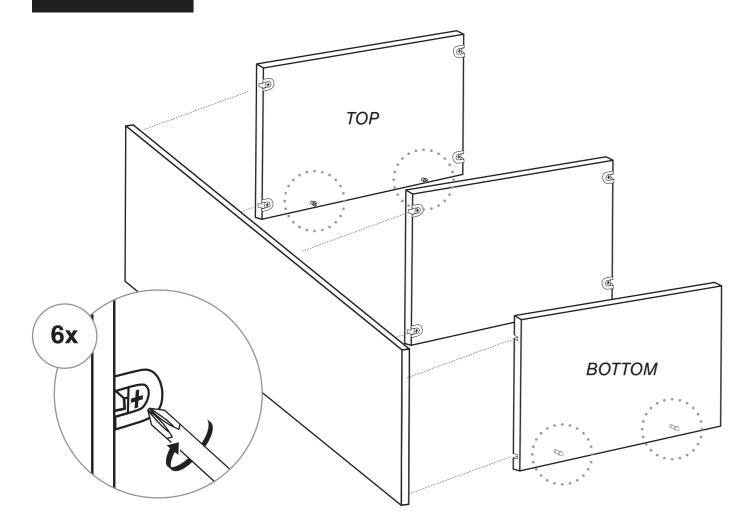
Note – the cam lock screws on the top and bottom panels should point to the inside of the cabinet.
