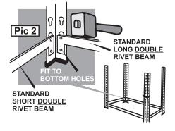
Fit remaining 2 Standard Long DOUBLE Rivet Beams and remaining 2 Standard Short DOUBLE Beams where you want the 4th Shelf to be positioned. (Pic 4)
