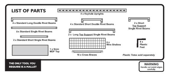
Attach a Plastic Foot to 1 end (bottom end) of each of the 4 Keyhole Uprights. NOTE: Ensure keyholes are the correct way up. (Pic 1)
