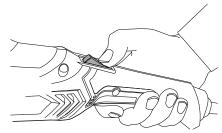
2. To turn OFF, release the On/Off rocker switch. The switch will return back into the off (0) position.
