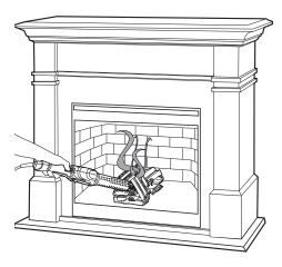
4. When the paper catches fire, slowly pull the charcoal starter 100 - 200mm away from the fire, while keeping it aimed at the same point until the twigs/kindling combust in the fireplace.
