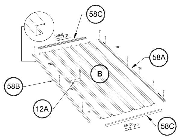
Vertical door channels are installed in the opposite orientation compared to the horizontal door channels.
