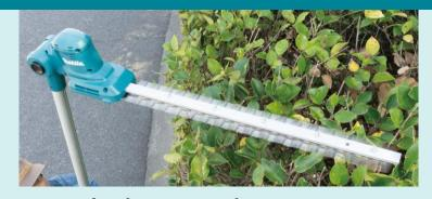
Blade Length: 460mm Max. branch diameter: 18mm
