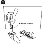
Install valve into the cistern and firmly tighten. Do not use a spanner.
