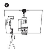
Remove filter from the base of the inlet.
