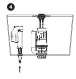
Re-install filter and connect water supply.
