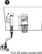
Turn off water supply before cleaning filter. Remove hose connection from the base of the valve
