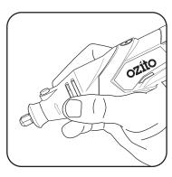
4 For heavy work like cutting or grinding, hold the rotary tool in the palm of your hand.
