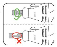
6 Tighten collet nut using spindle lock and spanner.
