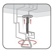
3 Screw the desk stand shaft into the hole at the top of the clamp.
