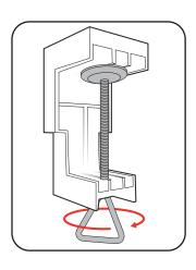
2 Place the desk stand clamp onto the desk and tighten the clamp.
