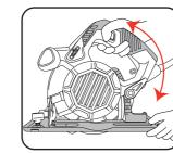
2. Hold the baseplate down with one hand. Raise or lower the saw to the desired depth, referring to the scale.
