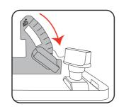
3. Confirm the angle between the blade and the baseplate is 90° using a square.
