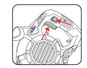
4. To stop the saw, release the on/off switch.
