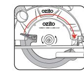
4. Remove and replace blade. Ensure arrows on the blade point in the same direction as the arrow on the upper blade guard.
