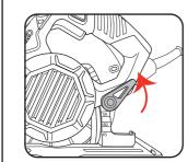
1. Loosen the depth adjustment knob.
