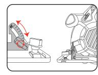
5. Tighten bevel adjustment
