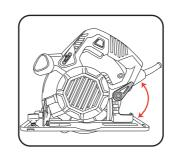
2. Loosen bevel adjustment knob. Set to 0° on the scale. Tighten bevel adjustment knob.
