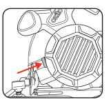
5. Fit outer blade flange and blade bolt. Depress spindle lock.
