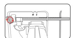
2. Set to desired width by aligning the scale with the cutting guide
