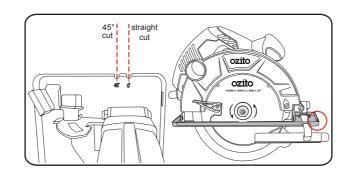
4. The cutting guide will give an approximate line of cut. For a straight cut, use the 0° notch. For a 45° cut, use the 45° notch.
