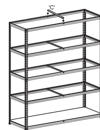
Apply remaining brackets as above to desired height. Ensure that braces 'C' are fixed to all shelves
