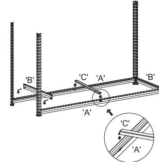
Use shelf bracket 'B' for the side brackets using the shelf bracket from Step 1 as a guide for height. Allow 1 keyhole free from the ground as shown in the diagram. Use same shelving brackets for opposing sides as shown in the diagram. Place brace 'C' as shown.
