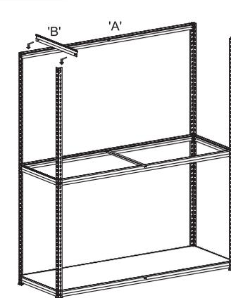
Fix brackets 'B' at the very top allowing room for the MDF board to sit flush against the legs. Repeat with brackets 'A'.
