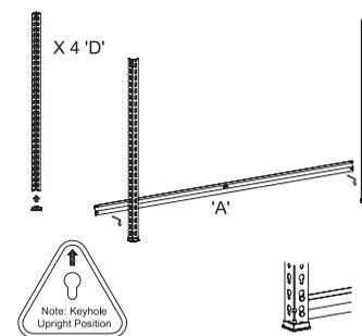
Allow one keyhole free between the foot cap and the shelving bracket.
