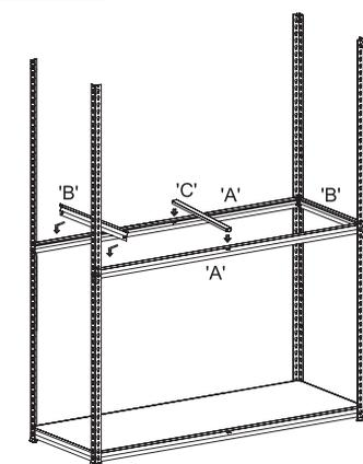
Fix brackets 'B' so that the top rivet sits on the upper legs and the bottom rivets sit on the lower legs. Repeat with brackets 'A', followed by brace 'C' as shown
