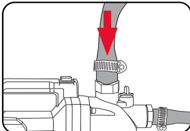
**Note:** The discharge hose or pipe you are using must have a minimum diameter of 13mm (1/2").
