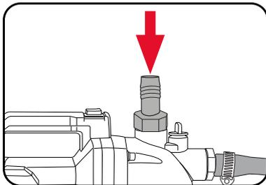
3. Securely attach the input hose or pipe to the other end of the adaptor. Ensure you have the correct diameter hose or pipe that is compatible with your water discharge application.
