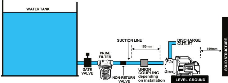
Connection with tank base below transfer pump
