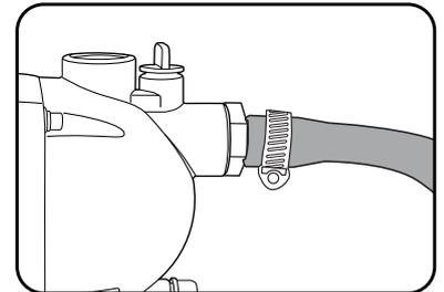
**Note:** The input hose or pipe you are using must have a minimum diameter of 25.4mm (1").
