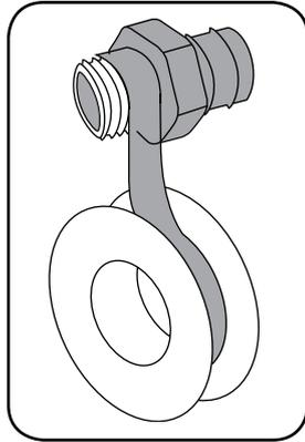
2. Remove the plastic protection cover from the discharge outlet and insert a 25.4mm (1") male threaded hose adaptor (not included). Tighten firmly with a spanner (not included).
