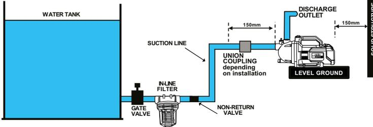
**Note:** A non-return valve is recommended so that the water does not run off when the pump is shut off.
