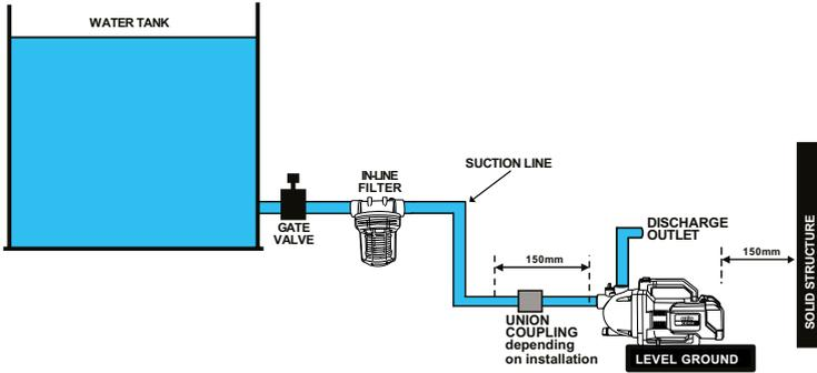
Connection with tank base level with transfer pump
