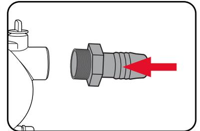
3. Securely attach the input hose or pipe to the other end of the adaptor. Ensure you have the correct diameter hose or pipe that is compatible with your water drawing source.
