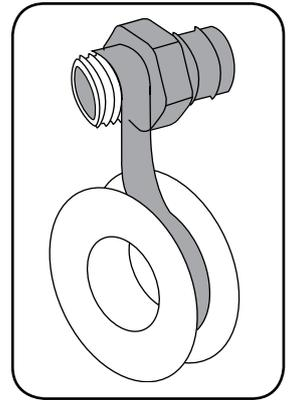
2. Remove the plastic protection cover from the suction inlet and insert a 25.4mm (1") male threaded hose adaptor (not included). Tighten firmly with a spanner (not included).
