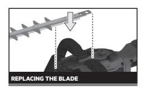
**NOTE:** Blades should be regularly sharpened or replaced to ensure the best cut quality and performance of the product.
