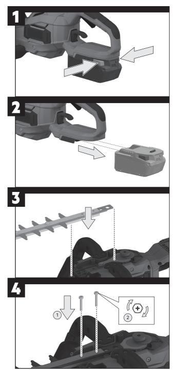
**NOTE:** Do not overtighten the bolt. The torque setting is 1.6-2.2 Nm.
