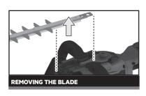
**NOTE:** Blades should be regularly sharpened or replaced to ensure the best cut quality and performance of the product.
