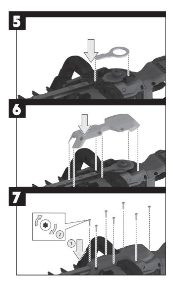
**NOTE:** Do not overtighten the bolt. The torque setting is 0.8-1.8 Nm.
