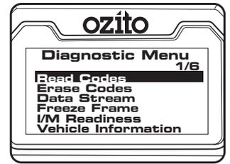
1. Use the “UP” and “DOWN” buttons to select a Read Codes and press the “OK” button to confirm.
