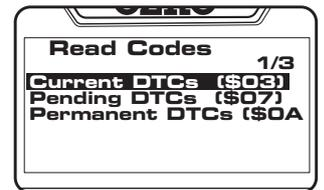
**PD (Pending) DTC codes-** They indicate problems that the control module has detected during the current or last driving cycle but are not considered serious yet. Pending Codes will not turn on the malfunction indicator lamp (MIL) unless the same problem is detected again. If the fault does not occur within a certain number of warm-up cycles, the code clears from memory.
