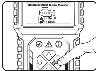
2. Wait for the menu to appear. A sequence of messages displaying the OBD2 protocols and progress bar will be observed on the backlit LCD until the vehicle protocol is detected.
