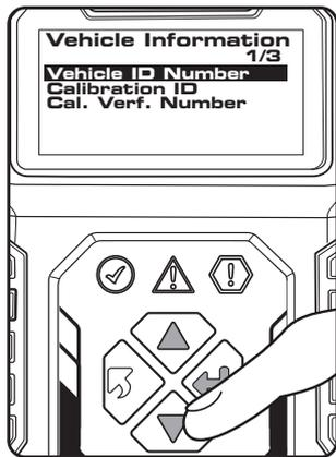
**Note:** If the vehicle does not support selected mode, a “Not Supported” message shows on the backlit LCD.
