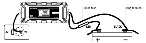
3. Fit the correctly rated fuse.
