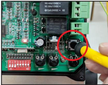
Press and hold the learn button (K4) until the Learn LED flashes ON.
