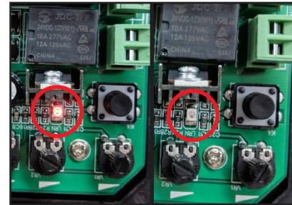
The Learn LED will flash repeatedly and then turn OFF. when the remote is paired.
