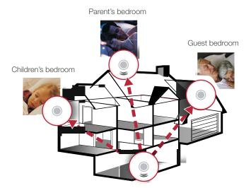
Interconnected alarm detects fire somewhere in the home and triggers other Quell interconnected alarms in the network.
