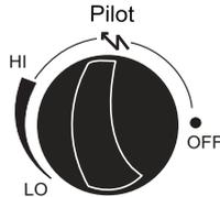
3. Activate the igniter button repeatedly until you see the blue flame of the pilot through the viewing hole in the mesh. The pilot flame can be difficult to see in direct sunlight.
