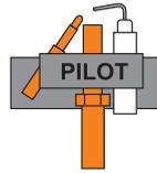
2. **To light the heater,** turn the control knob to the pilot position and keep the control knob depressed so gas can flow to the pilot burner. This can take up to 1 minute.
